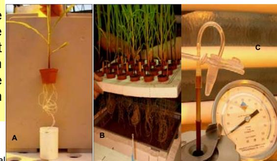
**Picture 1.** Horizontal split-roots system (45% in soil, 55% protruding the pots; A) making it possible to chill (8 °C) the lower part of the root in nutrient solution (B). Water potential was determined and xylem sap collected from freshly de-topped and pressurised roots of chilled and control maize seedlings by pressure chamber (C).
