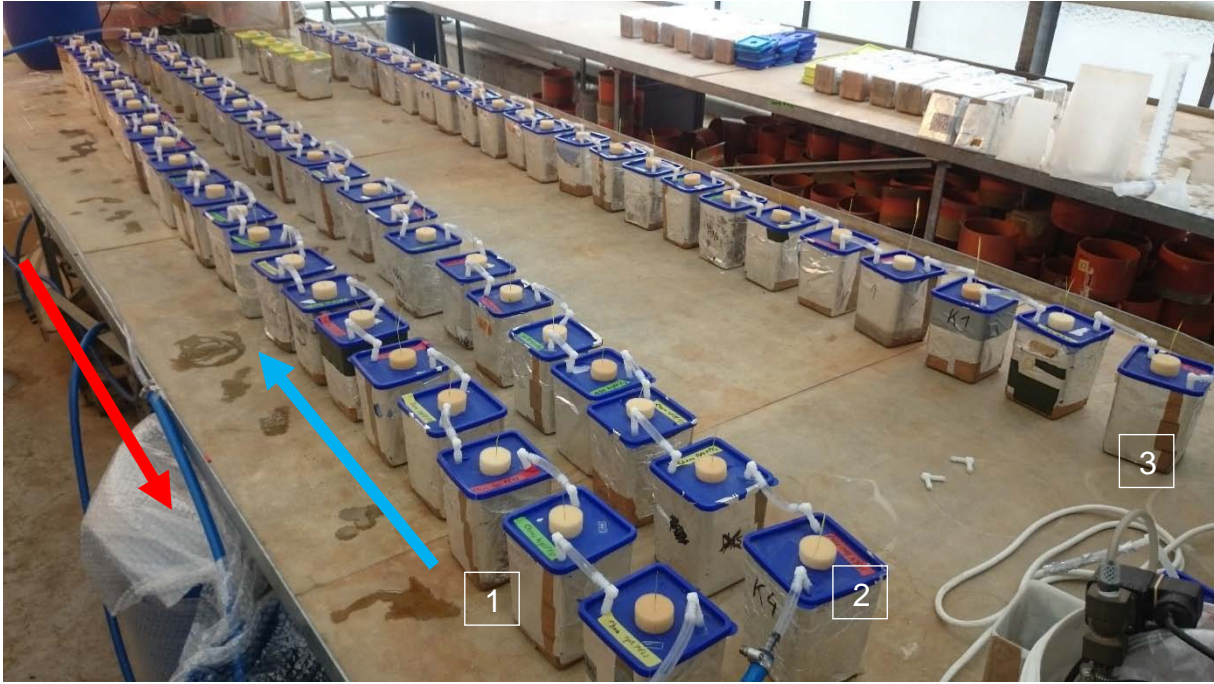
Figure 3: Experimental Setup of experiment 1 with three blocks for different root zone temperatures, blue arrows (cool) and red arrow (heated) shows cooling cycle. 1: low temperature; 2: medium temperature and 3: high temperature
