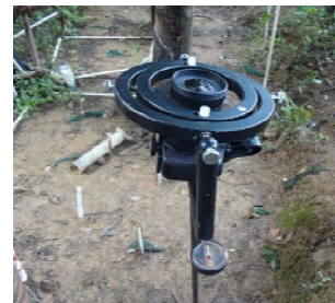
Hemispherical photography method HemiView Delta-T Devices Ltd, Cambridge, UK
